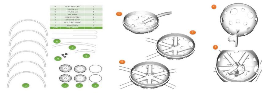
STEP 1: Place tubes in large hole of bottom cover one at a time while inserting 11" zip tie in tube holes. The rough side of the zip tie on the inside.
